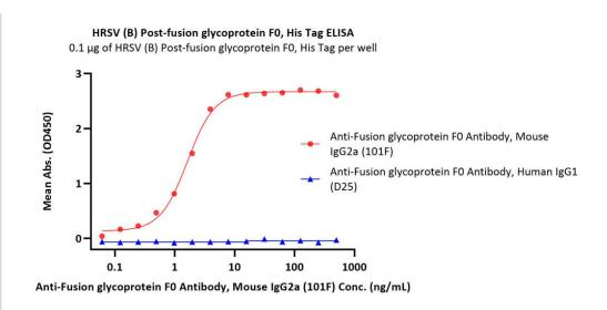
Immobilized HRSV (B) Post-fusion glycoprotein F0, His Tag (Cat. No. RSF-V52H9) at 1  $\mu$ g/mL (100  $\mu$ L/well) can bind Anti-Fusion glycoprotein F0 Antibody, Mouse IgG2a (101F) with a linear range of 0.1-4 ng/mL and not bind Anti-Fusion glycoprotein F0 Antibody, Human IgG1 (D25) (QC tested).
