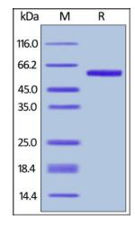
Biotinylated Human OX40 Ligand, Avitag,Fc Tag on SDS-PAGE under reducing (R) condition. The gel was stained with Coomassie Blue. The purity of the protein is greater than 95%.
