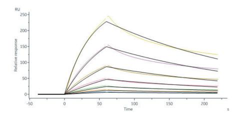
Human ITGA7X2B&ITGB1 Heterodimer Protein, His Tag&Tag Free (Cat. No. IT1-H52W8) immobilized on CM5 Chip can bind Human Laminin 221 Protein, premium grade (Cat. No. LA2-H5269) with an affinity constant of 49.8 nM as determined in a SPR assay (Biacore 8K) (Routinely tested).
