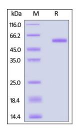
Human MMP-1 Protein, His Tag on SDS-PAGE under reducing (R) condition. The gel was stained with Coomassie Blue. The purity of the protein is greater than 95%.
