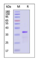
HRSV (A) Glycoprotein G Protein, His Tag on SDS-PAGE under reducing (R) condition. The gel was stained with Coomassie Blue. The purity of the protein is greater than 90% (With <u>Star Ribbon Pre-stained Protein Marker</u>).
