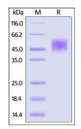
Rubella virus Glycoprotein E2 (strain M33) (RUBV), His Tag on SDS-PAGE under reducing (R) condition. The gel was stained with Coomassie Blue. The purity of the protein is greater than 90%.
